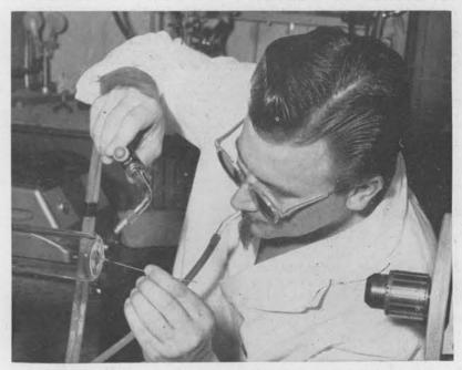
DELICATE TOUCH of Joe Chouinard, 1413, eases a wire filament into a vacuum tube being blown in the Physical Electronics Laboratory. Joe holds a flame torch to melt the glass and gently puffs through the tube to shape it into the desired form.
